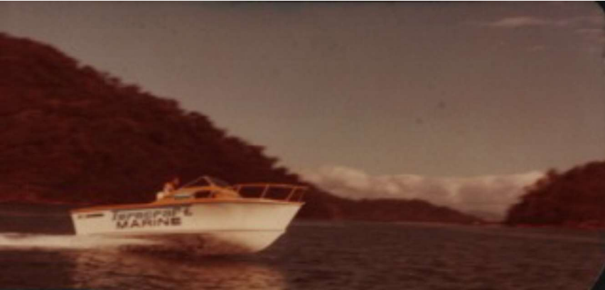
Photo...I designed and built this, Turncraft Marine.. 21foot Flared Bow Aluminium Boat (sterndrive)
