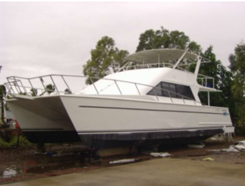
Photo...(centre) I designed and built this 50ft Power Catamaran (25 knts plus) with two 300 HP Yanmar diesels Photo below... I designed and built this 60ft Power Catamaran ( 27 knts plus) with two 450 HP Cummins diesels... tunnel hulls aft (props and rudder)
